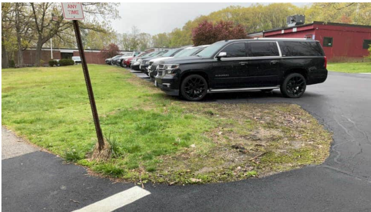
Opportunity to install bioretention planter at grassed corner where flow passes before reaching roadway. Additional opportunity exists to install infiltration trench along parking lot edge for additional treatment opportunity.
